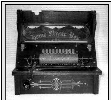
Figure 5. The 20-note Gem Roller Organ was manufactured by the Autophone Co. in Ithaca, NY. The machine plays a small wooden roller with the music arranged spirally with rows of small pins that open the metal valve levers as the roller rotates. The music lasts 43 seconds as the roller turns three rotations to the right and then returns to home position. Tens of thousands of the Gem organettes were made in the 1800s and early 1900s. Sears Roebuck Co. listed the Gem for $3.25 in their 1902 catalog.
